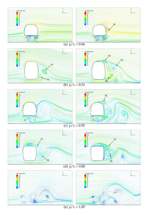
Figure 7: 2D streamlines at different locations on the *y*-axis, t=1s,  $\beta \approx 20.27^{\circ}$ . Left: CFX; Right: NKS.
