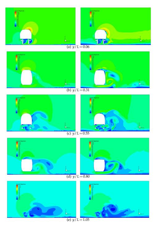
Figure 6: Velocity contours at different locations on the y-axis, t=1s,  $\beta \approx 20.27^{\circ}$ . Left: CFX; Right: NKS.
