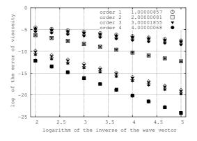
Figure 16: One point periodic analysis. Error  $\epsilon \equiv \mid \mu - \mu_{num} \mid$  between numerical and theoretical diffusivities. Four sets of parameters defined at relations (6.3), (6.4), (6.5), (6.6) and (6.7) lead to schemes of several orders. The measured orders with a linear regression are displayed in the right column.
