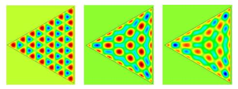
Figure 11: Dirichlet mode number "7" of an equilateral triangle (left) and errors for a D2T7 computation. The exact reference eigenvalue is equal to 108. The numerical eigenvalue is equal to 107.90777 at order 2 (middle) and to 107.92705 at order 4 (right). The  $L^{\infty}$  error for the modes with this computation is equal to  $1.02 \times 10^{-2}$  at order 2 and  $4.2 \times 10^{-3}$  at order 4.
