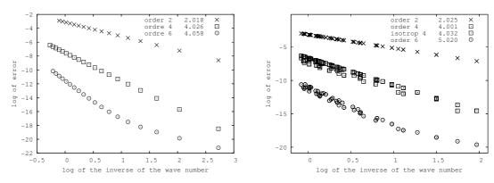
Figure 3: D2T7 lattice Boltzmann scheme for the heat equation. Periodic modes for a pipe with nx=96 and ny=4 mesh points (left) an periodic modes for a rectangle of nx=36 by ny=52 points (right). Error  $\epsilon\equiv \mid \mu-\mu_{\rm num}\mid$  between exact and numerical diffusivities. The hexahedric predicted coefficients define a fourth or fifth order scheme.
