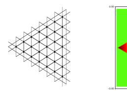
Figure 4: Typical two-dimensional mesh for a D2T7 computation on a triangle (left). Two-dimensional computation of the harmonic function  $p_H(x,y)=x^2-y^2$  on a triangle with the D2T7 lattice Boltzmann scheme (right). The iso-contours are composed by discrete hyperbolas.
