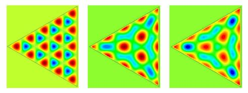
Figure 10: Isovalues of the Dirichlet mode number "5" of an equilateral triangle (left) and errors for a D2T7 computation. The exact reference eigenvalue is equal to 48. The numerical eigenvalue is equal to 47.98339 at order 2 (middle) and to 47.98842 at order 4 (right). The  $L^{\infty}$  error for the modes is equal to  $3\times 10^{-2}$  at order 2 and  $1.1\times 10^{-3}$  at order 4.
