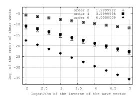
Figure 2: D2T7 lattice Boltzmann scheme for the heat equation. One point periodic analysis. Error  $\epsilon \equiv |\mu - \mu_{\text{num}}|$  between exact and numerical diffusivities. Note that the exact dispersion equation can be obtained, and when solved by successive approximations in powers of k, it leads to the same results, obtained from the successive equivalent equations.
