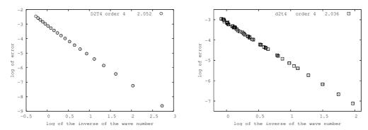
Figure 17: D2T4 lattice Boltzmann scheme for the heat equation. Periodic modes for a pipe with nx=96 and ny=4 mesh points (left) and a rectangle of nx=36 by ny=52 points (right). Error  $\epsilon\equiv \mid \mu-\mu_{\rm num}\mid$  between exact and numerical diffusivities. The predicted coefficients for the order 4 define a second order scheme in this particular case.
