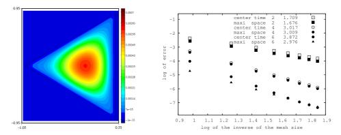
Figure 8: Dissipation of the first Dirichlet mode. Isocontours of the field of error at T=4/3 with a mesh composed by 61 points on the edge (left). Negative values in blue and positive ones in red. Time and  $L^{\infty}$  space errors for several meshes and several "orders" with the D2T7 lattice Boltzmann scheme. The obtained accuracy is not the one proposed by the Taylor expansion method. The space numerical accuracy is going from 1.7 to 3.0 with a good tuning of the numerical parameters.
