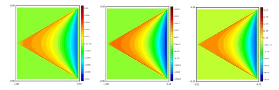
Figure 5: Two-dimensional computation of the harmonic function  $p_H(x,y)=x^2-y^2$  on a triangle with the D2T7 lattice Boltzmann scheme. Iso-contours of the errors for three sets of parameters presented at relations (3.6), (3.7) and (3.8). Negative values are in blue and positive ones in red. The maximal errors are equal to  $8.1410^{-4}$  (left),  $2.3610^{-4}$  (middle) and  $4.4710^{-5}$  (right) when using a D2T7 scheme with formal order of 2 (left), 4 (middle) and 6 (right).
