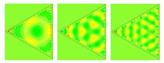
Figure 19: Isovalues of the errors for D2T4 computation of Dirichlet modes of an equilateral triangle. The exact reference eigenvalues are equal respectively to 12, 48 and 108 and the computed ones to 11.97493, 47.59816 and 105.95870. This figure can be compared to second order accurate D2T7 results at Figs. 9, 10 and 11 respectively.
