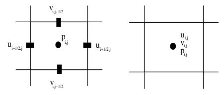
Figure 1: A solution representation on staggered versus non-staggered cells.
