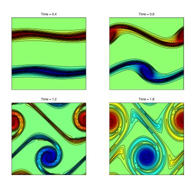
Figure 5: Vorticity solutions from the thin shear layer problem on  $128\!\times\!128$  mesh.
