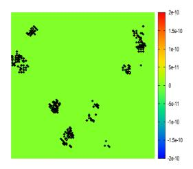
Figure 7: Divergence of the velocity field from the thin shear layer problem on  $128 \times 128$  mesh.
