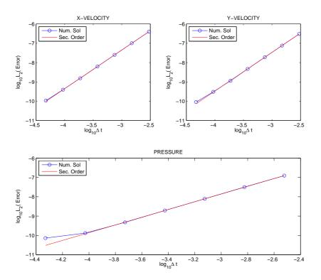
Figure 4:  $L_2$  norm of the time errors of the numerical solutions of the lid driven cavity problem on  $256 \times 256$  mesh at time = 0.5 and with Re = 1000.
