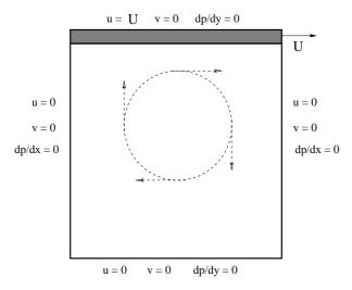
Figure 2: Lid driven cavity initial problem representation (lid is moving with a constant velocity U).
