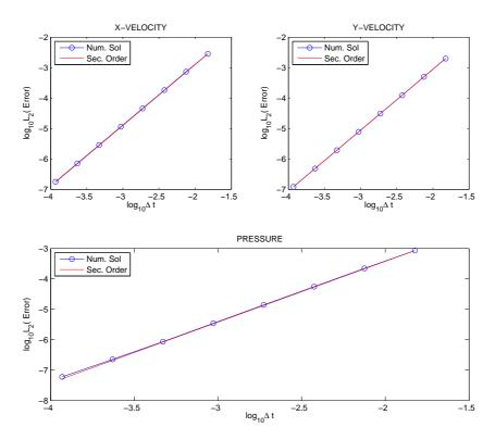
Figure 8:  $L_2$  norm of the time errors of the numerical solutions of the thin shear layer problem on  $256 \times 256$  mesh at *time* = 1.0.
