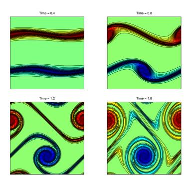
Figure 6: Vorticity solutions from the thin shear layer problem on  $256 \times 256$  mesh.
