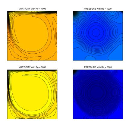
Figure 3: Steady state solutions of the lid driven cavity problem on  $256\times256$  mesh and for two different Reynolds numbers.
