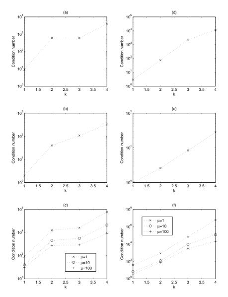
Figure 5: Condition number vs order for single element mass matrices, quasi-stiffness matrices and composite matrices for 1-form bases ((a), (b), (c )) and 2-form bases ((d), (e), (f)) on hexahedra.
