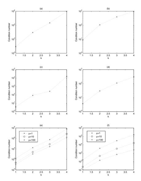
Figure 6: Condition number vs order for single element mass matrices (a), (b), quasi-stiffness matrices (c), (d) and composite matrices (e), (f) for B and C-type 1-form bases on prisms.
