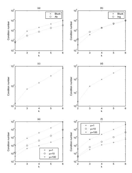
Figure 3: Condition number vs order for single element mass matrices (a), (b), quasi-stiffness matrices (c), (d) and composite matrices (e), (f) for B and C-type 1-form bases on tetrahedra respectively.
