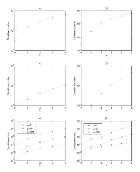
Figure 4: Condition number vs order for single element mass matrices (a), (b), quasi-stiffness matrices (c), (d) and composite matrices (e), (f) for B and C-type 2-form bases on tetrahedra respectively.
