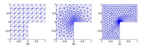
Figure 5: The *L*-shaped domain meshes used in simulations. The uniform mesh on the left consists of 65 vertices and 96 elements. The lightly refined non-uniform mesh on the center consists of 233 vertices and 422 elements. The densest non-uniform mesh on right consists of 704 vertices and 1304 elements.
