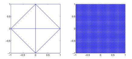
Figure 2: The computational domain is  $[-1,1] \times [-1,1]$ . The coarsest (h=1.0) and densest (h=0.03125) meshes for the rectangular domain. Meshes are derived from the coarse mesh by uniform subdivision.
