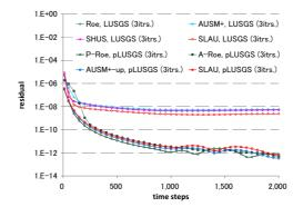
Figure 7: Residual histories, Case 2B ( $M_{\infty} = 0.01$ , inviscid), 3 sub-iterations.
