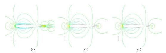
Figure 5: Computed flow fields ( $-1 < C_p < 1$ ), no sub-iterations, Case 2B ( $M_{\infty} = 0.01$ , inviscid): (a) LU-SGS/Roe (Unphysical), (b) LU-SGS/SLAU (Stable, slow convergence), and (c) pLU-SGS/SLAU (Stable, fast convergence).
