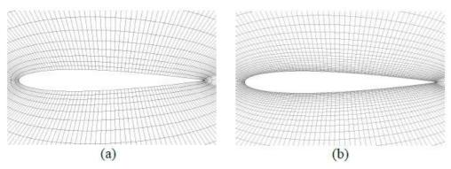
Figure 2: Computational grids for (a) inviscid ( $201 \times 31$  points) and (b) viscous ( $201 \times 51$  points) simulations.
