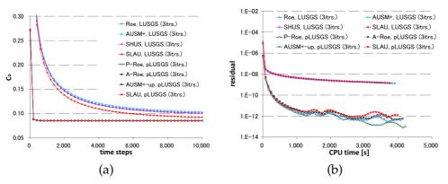
Figure 9: Drag coefficient and residual histories, Case 3 ( $M_{\infty} = 0.01$ , viscous), 3 sub-iterations: (a)  $C_D$ , (b) Residual.
