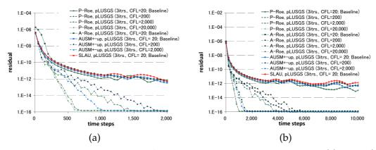
Figure 10: Residual histories with different CFL numbers for  $M_{\infty} = 0.01$ , 3 sub-iterations: (a) inviscid (Case 2B) and (b) viscous (Case 3) computations.
