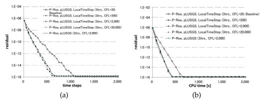
Figure 13: Residual histories with different CFL numbers, with and without local time stepping, for  $M_{\infty} = 0.01$ : (a) inviscid (Case 2B) and (b) viscous (Case 3) computations.
