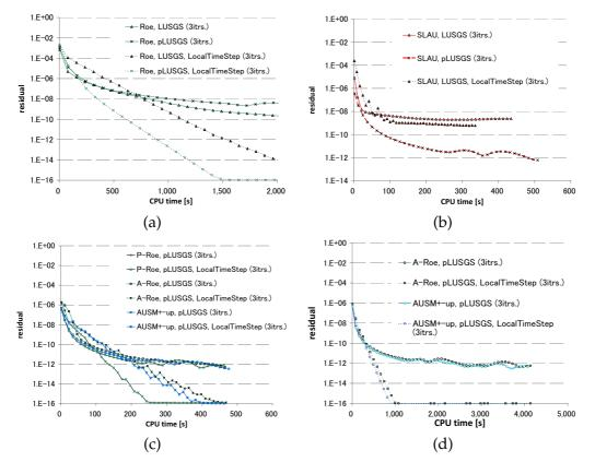
Figure 12: Residual histories with different CFL numbers, with and without sub-iterations: (a) viscous,  $M_{\infty} = 0.5$  (Case 1), (b), (c) inviscid,  $M_{\infty} = 0.01$  (Case 2B), and (d) viscous,  $M_{\infty} = 0.01$  (Case 3) computations.
