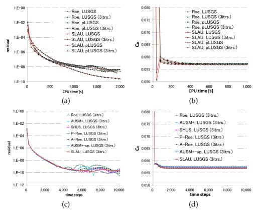
Figure 4: Residual and drag coefficient histories, Case 1 ( $M_{\infty} = 0.5$ , viscous): (a) Residual vs. CPU time, (b)  $C_D$  vs. CPU time, (c) Residual vs. time steps, and (d)  $C_D$  vs. time steps.
