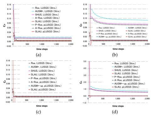
Figure 6: Drag coefficient histories, Case 2 (inviscid), 3 sub-iterations: (a) Case 2A ( $M_{\infty} = 0.1$ ), (b) Case 2B ( $M_{\infty} = 0.01$ ), (c) Case 2C ( $M_{\infty} = 0.001$ ), and (d) Case 2C ( $M_{\infty} = 0.001$ , wider scale for vertical axis).
