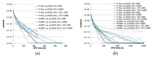
Figure 11: Residual histories with different CFL numbers, with and without sub-iterations, for  $M_{\infty} = 0.01$ : (a) inviscid (Case 2B) and (b) viscous (Case 3) computations.
