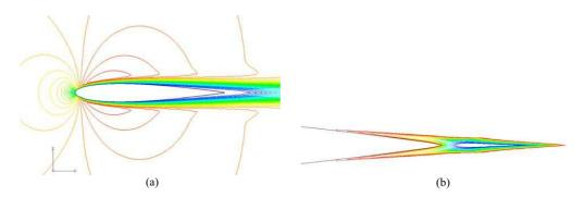
Figure 3: Computed flow field by LU-SGS/SLAU, no sub-iterations, Case 1 ( $M_{\infty} = 0.5$ , viscous): (a) Iso-Mach-contours (0 < M < 0.59), (b) *u*-velocity contours; blow-up view of separation region near the trailing-edge (-0.01 < u < 0).
