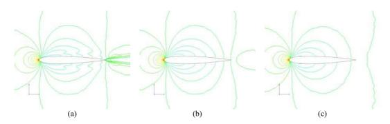
Figure 8: Computed flow fields ( $-1 < C_p < 1$ ), 3 sub-iterations, Case 3 ( $M_{\infty} = 0.01$ , viscous): (a) LU-SGS/Roe (Unphysical), (b) LU-SGS/SLAU (Stable, slow convergence), and (c) pLU-SGS/SLAU (Stable, fast convergence).
