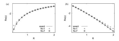
Figure 1: Comparison of the exact resonant values for a spheroid with the ones calculated within our approach for different N and an incident field oriented along the x-axis (a) and the z-axis (b). In the later Fig. 4, where we show the polarizability of a spheroids, the dependence of the resonant values on N can be seen in more detail.
