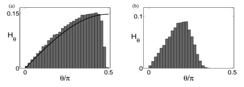
Figure 7: Histogram of the orientation (relative to  $E_{ext}$ ) of the induced dipole moment for all resonances (a) and only the biggest ones (b). The solid line in (a) is obtained if the orientation of the dipole axis is entirely random.
