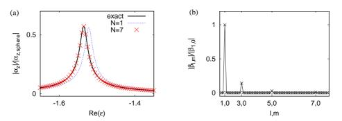
Figure 4: (Color online) Comparison of the exact and numerically calculated polarizability of a spheroid with R = 0.8 (a). The polarizability is normalized to the one of a sphere with radius 1 and a dielectric function of -2+0.01i. In the right panel (b) the coefficients of the spherical harmonics are presented for N=7 and a value of  $\epsilon$  close to the resonant value.
