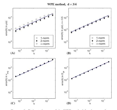
FIGURE 5. Estimated errors of the WPE method for the case of d = 3/4. (A) error in the probability density  $\rho(x)$ , (B) error in the probability density  $\rho(x)$  away from the discontinuity, (C) error in the average velocity, and (D) error in the effective diffusion. In four panels, solid lines are plots of  $y = c_1 h$  to show the order of convergence. It is clear that when the potential has a discontinuity at a half grid point, the WPE method has first order accuracy.
