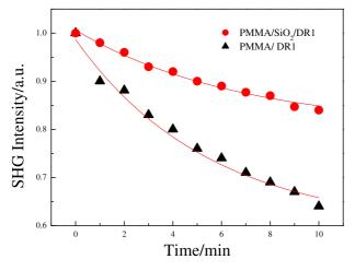
Figure 7: Relaxation of PMMA/DR1 film and PMMA/SiO<sub>2</sub>/DR1 film.
