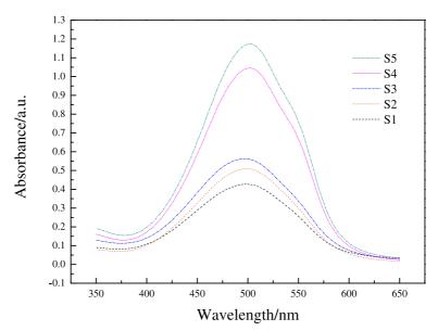
Figure 4: Absorption spectrum at different thickness of  $PMMA/SiO_2/DR1$  film.
