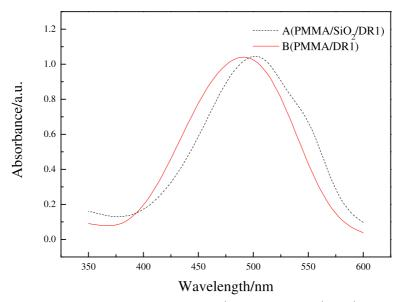
Figure 3: Absorption spectrum of PMMA/DR1 and PMMA/SiO $_2$ /DR1 film.
