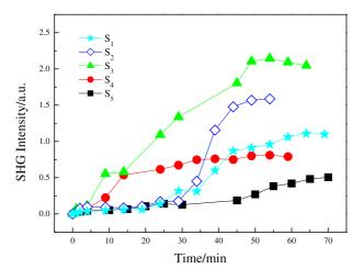
Figure 5: Dependence of SHG intensity on poling time at different thickness.
