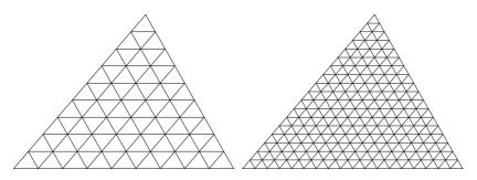
Fig. 4.2. The triangular meshes for the triangular domain  $\Omega$  (left: N = 9, right: N = 18).
