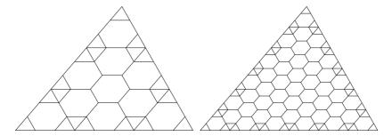
Fig. 4.1. The hexagonal meshes for the triangular domain  $\Omega$  (left: N = 9, right: N = 18).
