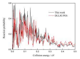
Fig. 3: The total reaction probabilities of the  $O + O_2$  reaction based on present PES and DLLIG PES, respectively, at total angular momentum J = 0 in the collision energy range from 0 to 0.5 eV.
