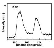
Figure 2. (a) XPS survey spectrum for amorphous Co-S-O and (b) Co 2p, (c) S 2p.
