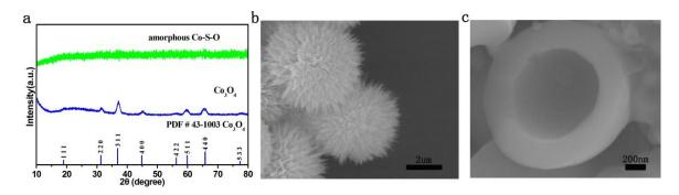
Figure 1. (a) XRD patterns of amorphous Co-S-O, and Co<sub>3</sub>O<sub>4</sub> precursor; (b) The SEM images of the Co<sub>3</sub>O<sub>4</sub> precursor; (c) The SEM images of the amorphous Co-S-O.
